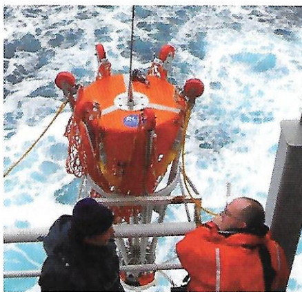
Figure 37: RLS – Rescue Star in stand-by position in a ring holder, after removal of the tarpaulin
